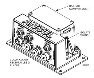
The protective battery compartment cover is held in place with 4 captive screws. Besides the internal power supply, the battery compartment includes the battery cable, a mini USB connection port, and the programming interface (button and LEDs). The system programming may be accomplished with the manual programming button and indicator LEDs or by using a computer with the ANSUL CHECKFIRE 210 Programmer software communicating through the mini USB port.
